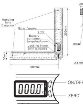
**ON/OFF** Short press ON/OFF to turn on the device. Short press ON/OFF to shut off the LCD. Long press ON/OFF for more than 3 seconds to shut off the whole system. Automatically shut off function in 6 min. Move the scale to turn on the device when at off LCD status.
